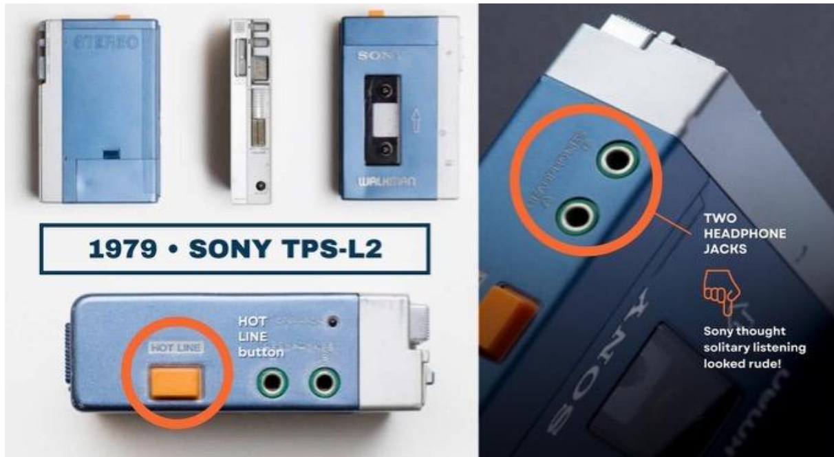
Figure 1. The Sony TPS-L2 Walkman featured two headphone jacks and a “hot line” button.
